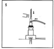
Slide the black 1/8" x 51/2" heat-shrink tubes on the bus wires, and the green/ yellow 1/4" x 51/2" heat-shrink tube on the ground pigtail. Heat shrink, using a heat gun, or soft flame torch, moving the heat source back and forth.
