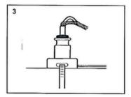
Extend the heater 71/2" above the base. Slide the grommet over the heater inserting the grommet in the base. Strip outer jacket 7" from end. Attach the base to the pipe with a pipe strap. (See Heat Trace Stripping Instructions for details.)
