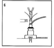
Slide the white ½" x 1½" heat-shrink tube in place over the bus wires and onto the inner jacket. Heat shrink in place. After removing the heat source, and while still hot, pinch the center of the heat-shrink tube between the bus wires with needlenose pliers.
