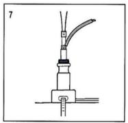
Make sure the sealing grommet is set in the base.
