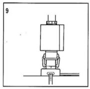
Mount junction box with non-threaded opening for 3/4" conduit, using the sealing gasket and lock ring to hold in place, or use a junction box with a 3/4" inside threaded hub.
