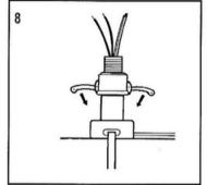
Slide the top in place and push and lock the cam levers into position. Lock cam levers by inserting the stainless steel tie wire through the holes in the ends of the cam levers and twisting together.
