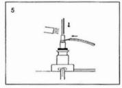
Slide the black 1/6" x 51/b" heat-shrink tubes on the bus wires, and the green/ yellow 1/4" x 51/b" heat-shrink tube on the ground pigtail. Heat shrink, using a heat gun, or soft flame torch, moving the heat source back and forth.
