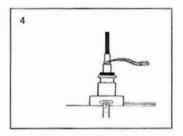
Strip the inner jacket 6" from the end. Strip the bus wires out of the core, following the Heat Trace Stripping Instructions.
