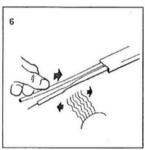
Slide the 1/s" x 5'/z" heat-shrink tubes on the bus wires. Shrink the tubes with heat gun or soft flame torch.
