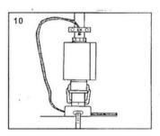
Mount junction box with non-threaded opening for 3/4" conduit, using the sealing gasket and lock ring to hold in place, or use a junction box with a 3/4" inside threaded hub. Ground the braid pigtail to conduit with a clamp (not provided).
