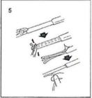
Notch the center core between the conductors and pull the bus wires away from the core for 6". Remove the center core material and any core material on the bus wires. Retwist the bus wires, if needed.
