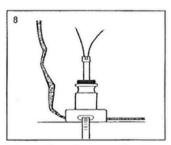
Make sure the sealing grommet is set in the base.
