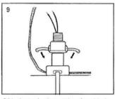
Slide the top in place and push and lock the cam levers into position. Lock cam levers in place by inserting the stainless steel tie wire through the holes in the ends of the cam levers and twisting together.
