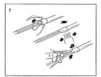
Slide the 1/2" x 11/2" heat-shrink tube over the bus wires and partially over the inner jacket. Heat shrink the tube; while still hot, pinch the center of the heat- shrink tube between the bus wires with needle-nose pliers.
