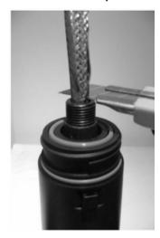
8. Wrap tape around the braid 1" (25 mm) from the end of the cut back outer jacket.
