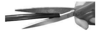
Trim the braid back to the edge of tape. Do not damage inner core.
