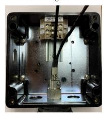
12. Tighten screw to securely capture the ground braid. Ensure good ground contact.
