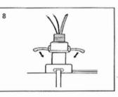
Slide the top in place and push and lock the cam levers into position. Lock cam levers by inserting the stainless steel tie wire through the holes in the ends of the cam levers and twisting together.
