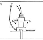
Slide the top in place and push and lock the cam levers into position. Lock cam levers in place by inserting the stainless steel tie wire through the holes in the ends of the cam levers and twisting together.
