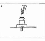
Extend the heater 7<sup>1</sup>/<sub>2</sub>" above the base. Slide the grommet over the heater inserting the grommet in the base. Strip outer jacket 7" from end. Attach the base to the pipe with a pipe strap. (See Heat Trace Stripping Instructions for details.)
