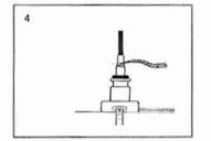
Strip the inner jacket 6" from the end. Strip the bus wires out of the core, following the Heat Trace Stripping Instructions.
