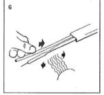
Slide the  $1/e^{\alpha} \times 5^{1}/e^{\alpha}$  heat-shrink tubes on the bus wires. Shrink the tubes with heat gun or soft flame torch.
