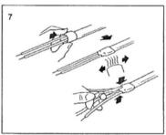
Slide the <sup>1</sup>/<sub>2</sub>" x 1<sup>1</sup>/<sub>2</sub>" heat-shrink tube over the bus wires and partially over the inner jacket. Heat shrink the tube; while still hot, pinch the center of the heat- shrink tube between the bus wires with needle-nose pliers.
