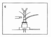
Slide the white ½" x 1½" heat-shrink tube in place over the bus wires and onto the inner jacket. Heat shrink in place. After removing the heat source, and while still hot, pinch the center of the heat-shrink tube between the bus wires with needlenose pliers.
