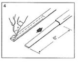
Strip the jacket 6" from the end to expose the conductive core.
