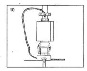
Mount junction box with non-threaded opening for  $3/a^{m}$  conduit, using the sealing gasket and lock ring to hold in place, or use a junction box with a  $3/a^{m}$  inside threaded hub. Ground the braid pigtail to conduit with a clamp (not provided).
