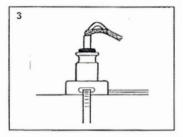
Make an opening in the ground braid, bend the heater, and pull the inner jacket and core through the opening in the braid. Twist the ground braid into a pigtail.
