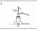
Slide the black  $\frac{1}{2}$ " x 5 $\frac{1}{2}$ " heat-shrink tubes on the bus wires, and the green/ yellow  $\frac{1}{4}$ " x 5 $\frac{1}{2}$ " heat- shrink tube on the ground pigtail. Heat shrink, using a heat gun, or soft flame torch, moving the heat source back and forth.
