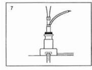
Make sure the sealing grommet is set in the base.
