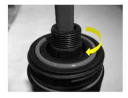
7. Install the Strain Relief (push on) over the cable and tighten the Clamp Screw. Cut and remove the outer jacket and braid to the top of the strain relief. Do not cut through to inner jacket.
