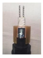
Note: It is very important the spacer (HXR) and core (LXR & MXR) be cut flush to the tape, between the bus wires, to ensure the WAGO Splice sits flush with the core (tape).
