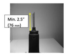
6. Tighten Connector until it bottoms out in order to compress the Grommet assembly.
