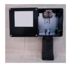
The  $\Omega$  HTS ACSX-1 Heat Trace Power Connection Kit is a CSA/(CUS) certified component for installation with  $\Omega$  HTS's Self-Regulating Heating Cables – LXR, MXR & HXR. The ACSX-1 connects a  $\Omega$  HTS Heater Cable to power and consists of a pipe mounted Stanchion and a J-Box complete with a DIN rail mounted terminal blocks.
